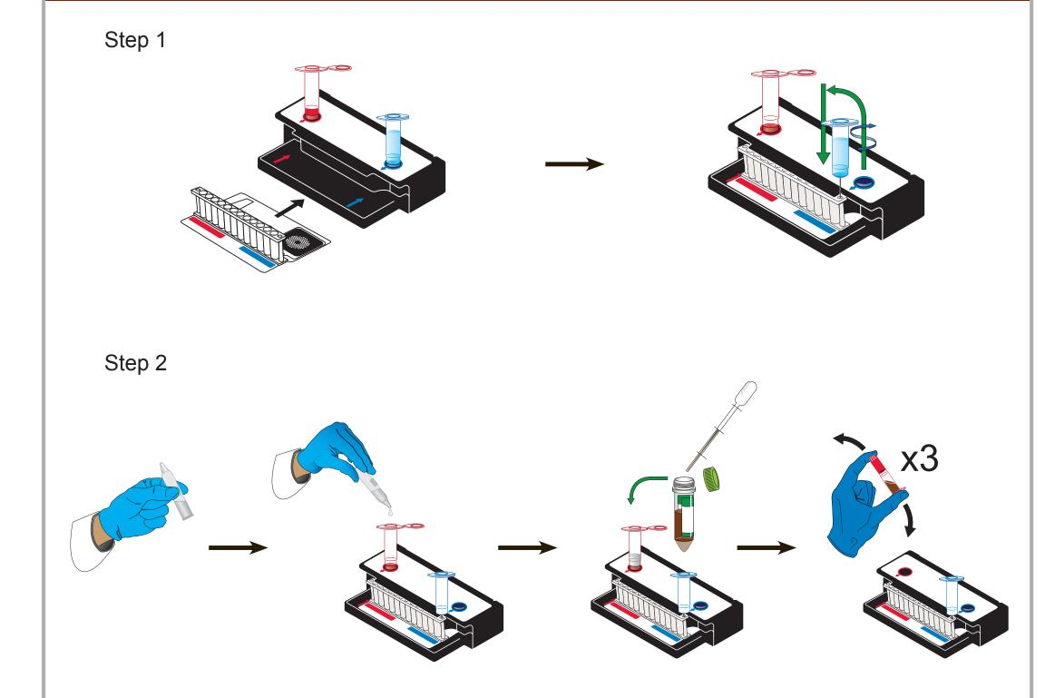
Testing of stool samples with the FilmArray GI Panel requires minimal pre-processing of specimens. The stool is diluted in Cary Blair medium (1:4) and loaded into the FilmArray GI pouch using a novel filter-injection vial. The user enters the sample and pouch type (using a barcode reader) into the software and initiates a run. The result of the test is ready in about one hour.
