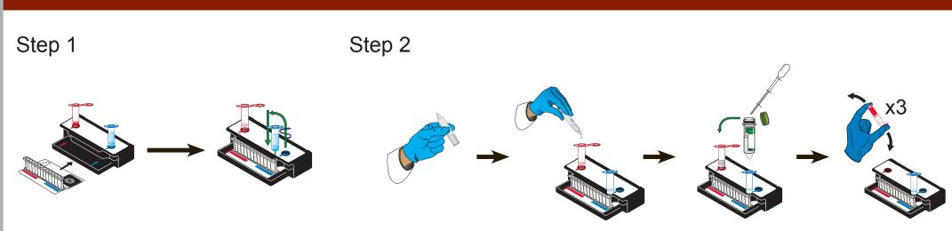
Testing requires minimal pre-processing of specimens. Cerebrospinal fluid and FA Sample Buffer are combined in a novel filter-injection vial (FAIV) and then loaded into the FA ME pouch. The user enters the sample and pouch type (using a barcode reader) into the software and initiates a run.
